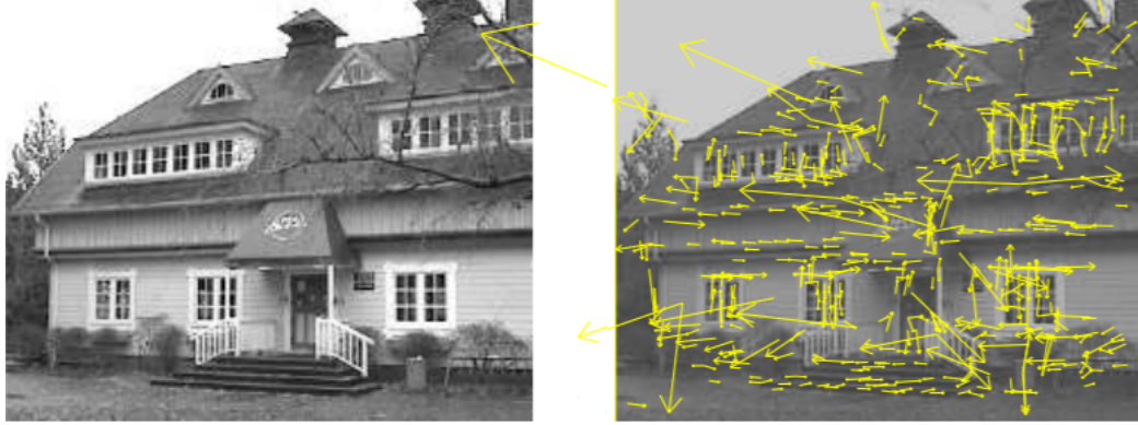
Figure 6: Illustration of the output of SIFT's keypoint extraction. Each keypoint is represented by a vector to visualize its scale, rotation, and position. 6
