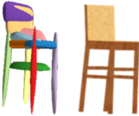
Figure 24: On the left is the superquadric decomposition of the original 3D model displayed on the right. Each of the 11 parts is uniquely colored.
